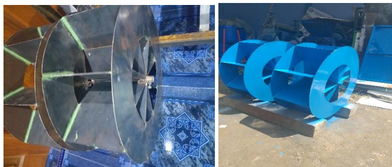
Gambar 2. Desain kincir air model kanal Overshot.
