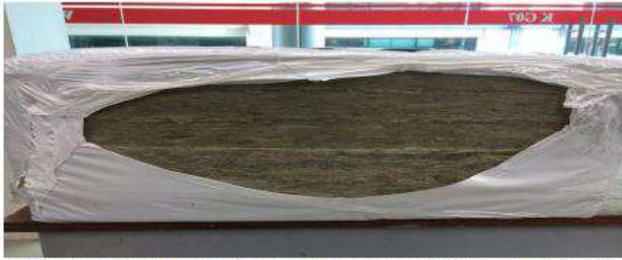
Fig. 1. Rockwool packed with 6 layers and thickness of 50 mm per layer
